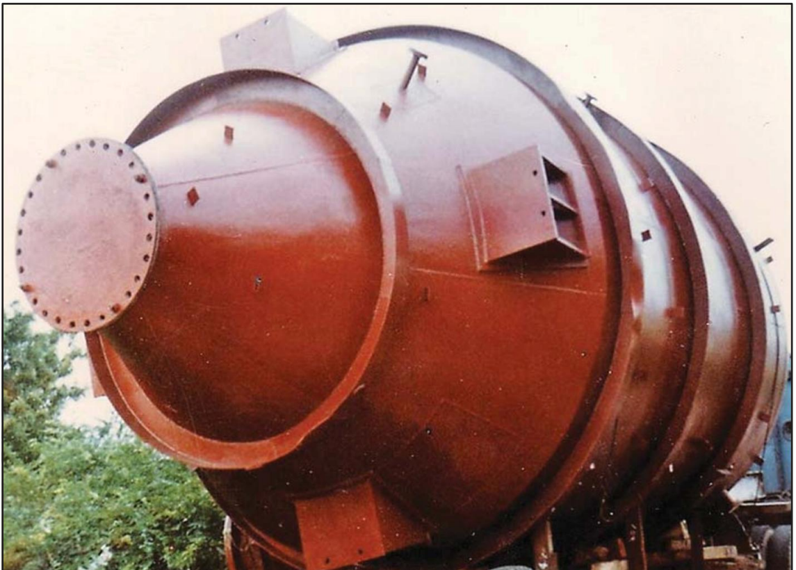
Rubber Lined Flash Chamber
